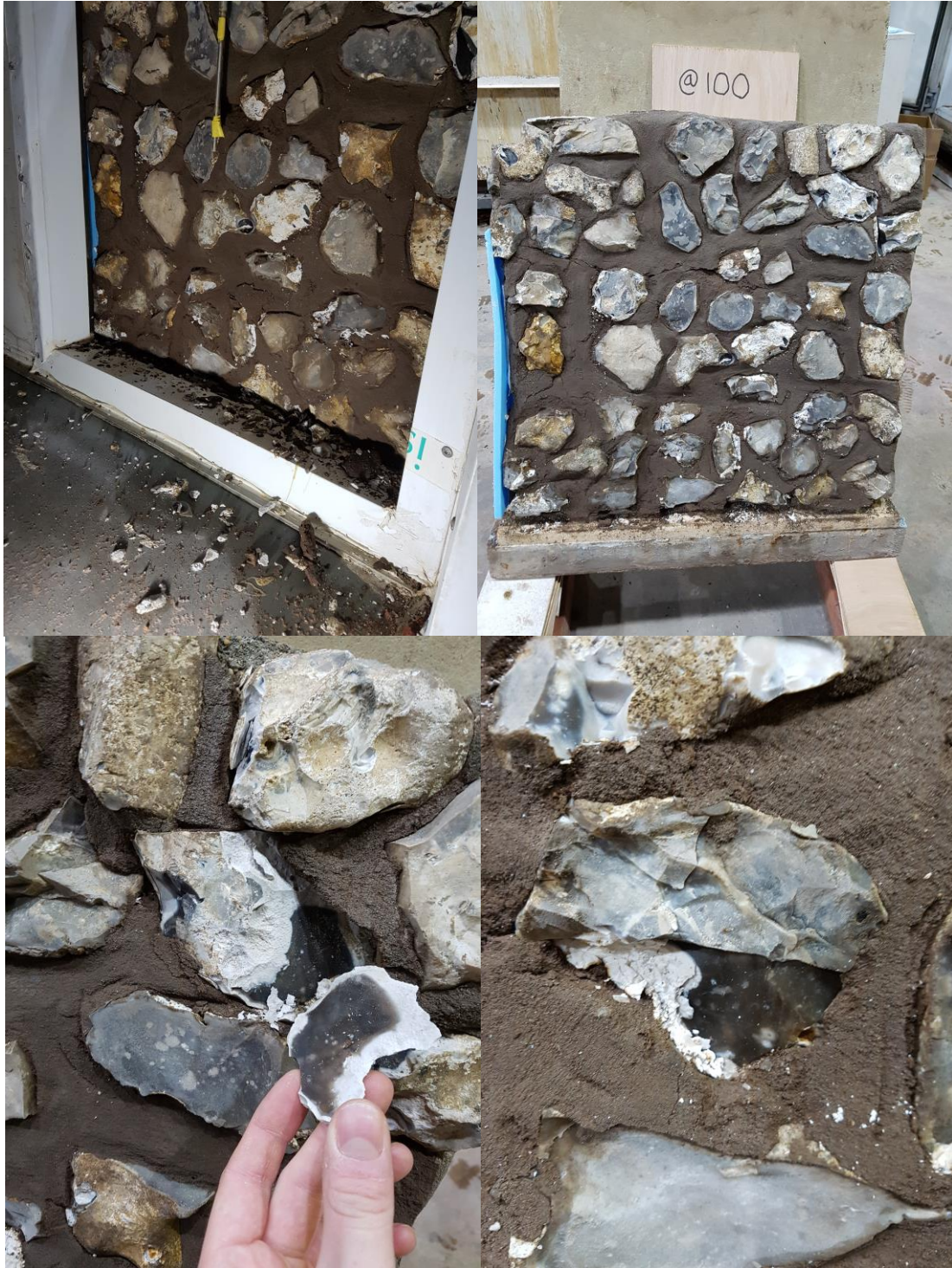
Figure 2 – Images of damage at 50 cycles and at 100 cycles at the end of the test.
